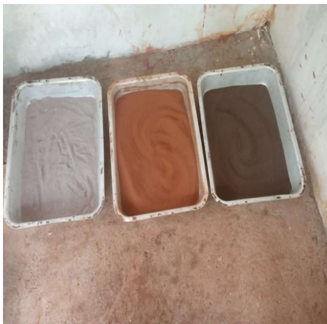
Fig -2: Sieved Boiler Ash, Soil and Sludge
