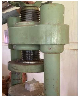
Fig – 10 : Compression testing
