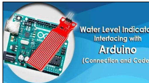
Figure 5: Drip level Sensor.
