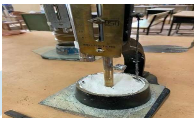
Fig 4. Consistency test on gypsum
