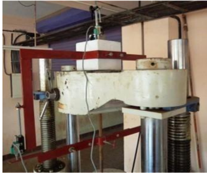
Fig.5. Pull out test setup
