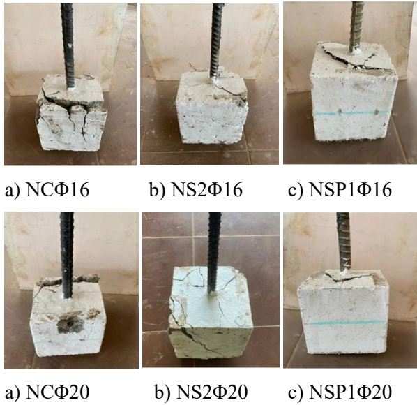
Fig. 11. Pull out failure
