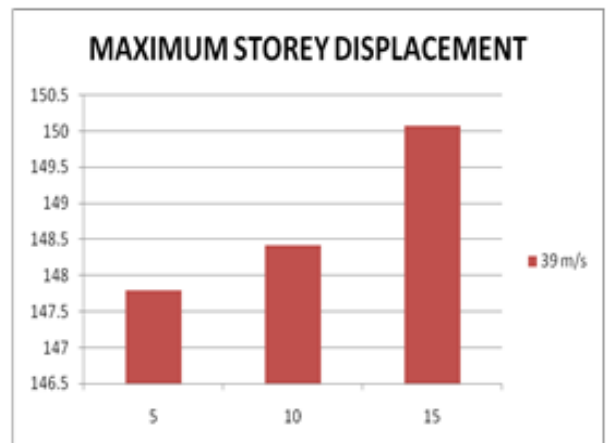
Fig. 6. Maximum storey displacement for wind velocity 39m/s
